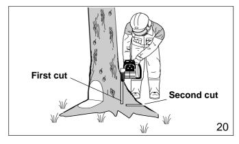
If the tree has large buttress roots, cut into the largest buttresses vertically first (horizontally next) and remove (fig. 20).
